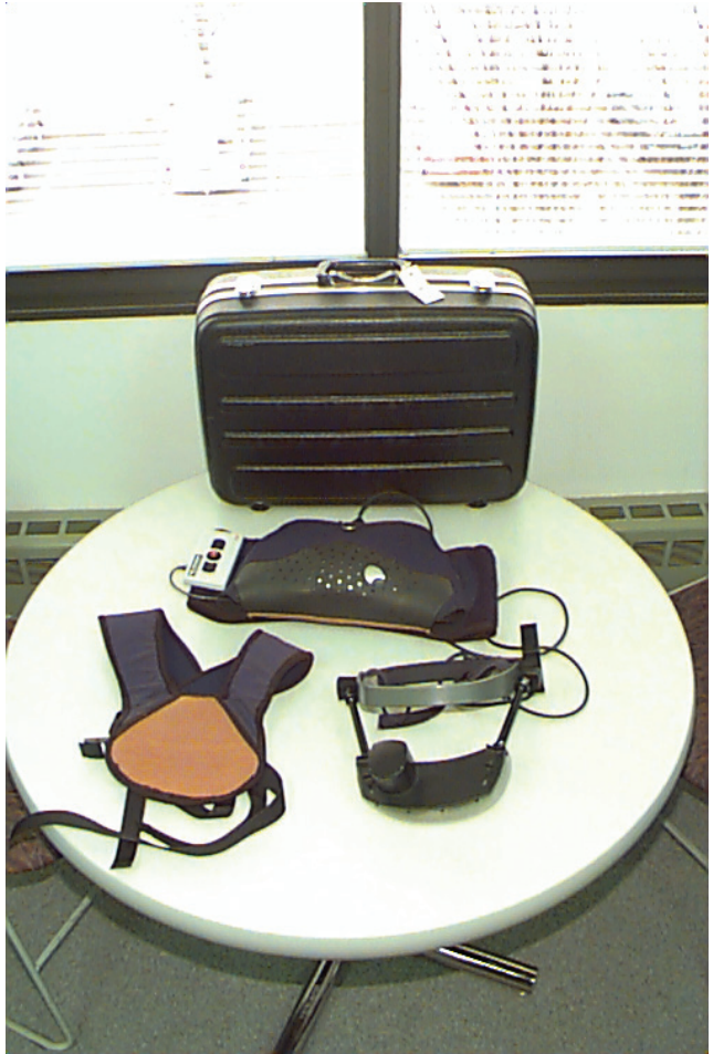
Figure 4.1.5 Wearable Computer with Case
