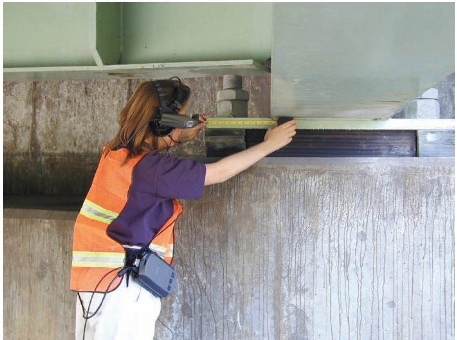
Figure 4.1.6 Inspector Using Wearable Computer
